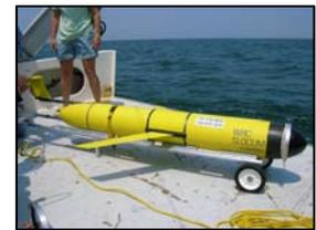
a few feet in length, AUVs can be packed with sensors, measuring anything from salinity and temperature to chlorophyll; some can even identify fish.
